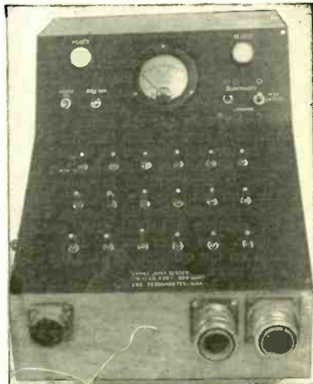
Special cables for production checking are fitted to the checker's three receptacles.
